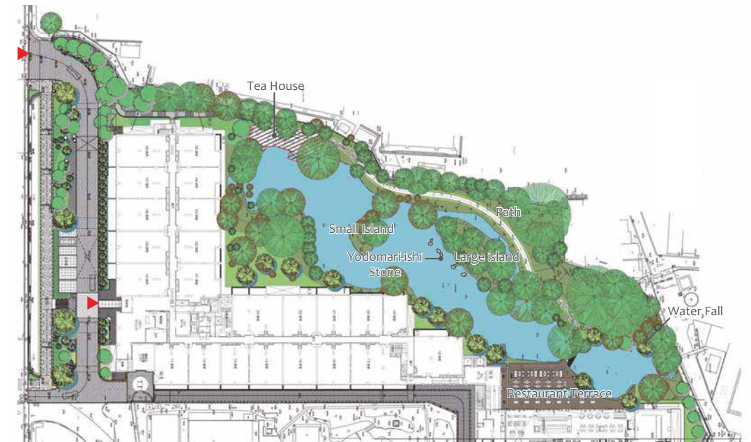
Restoration of the Water Fall A cascade restored with rearranged existing stones and relocated water source from a well.
